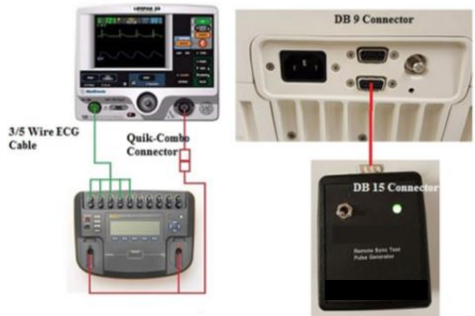
Figure 1.19: Quik-Combo Sync Remote Test Setup
