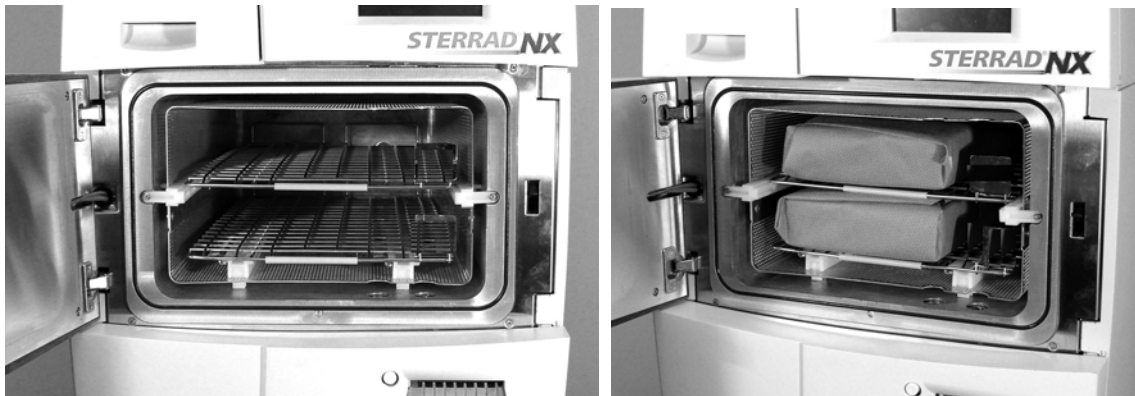
Figure 4. The STERRAD® NX™ Chamber Empty and With the Load Correctly Place.
