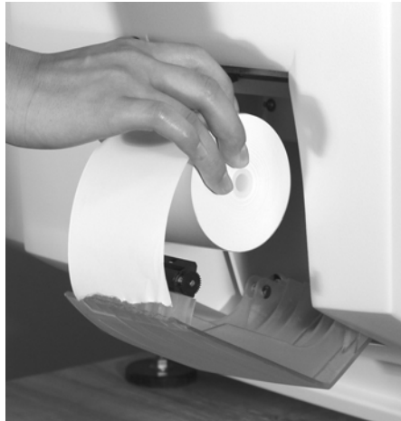
Figure 48. Insert a New Paper Roll.
