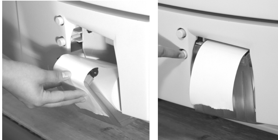
Figure 50. Hold the Paper as You Shut the Printer Door. Press the Paper Advance Button.
