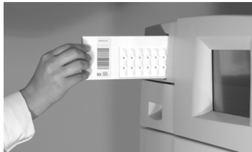
Figure 11. Inserting the Cassette into the Slot.
