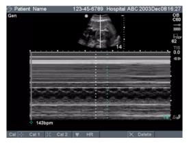
Figure 2 M Mode Trace Image with Heart Rate
