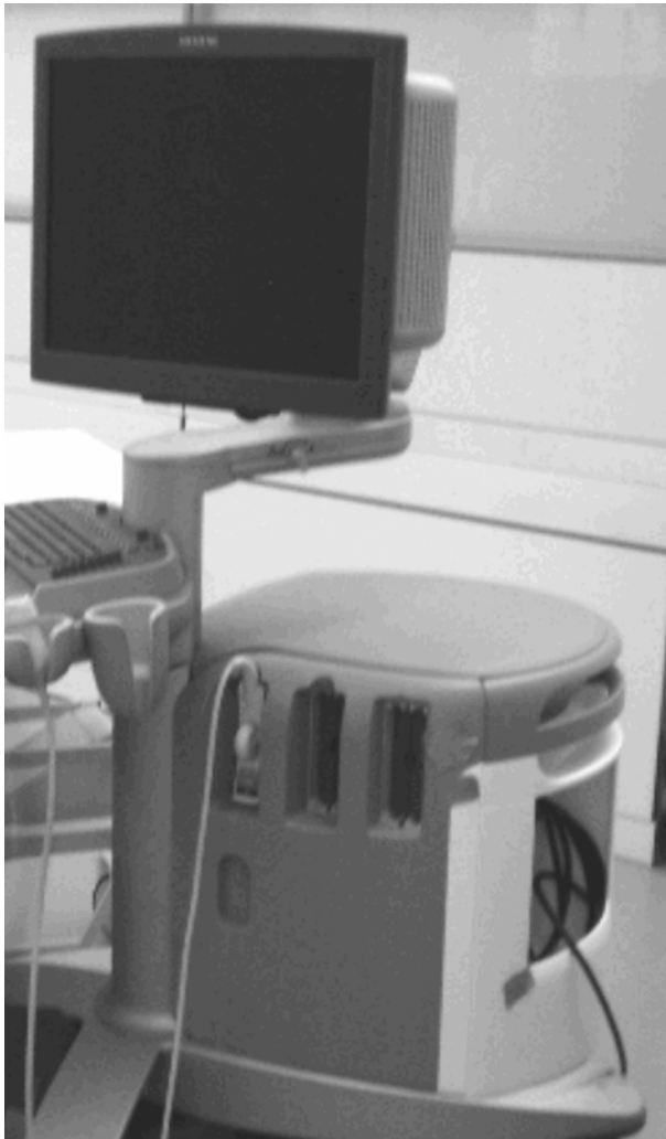
Fig. 15: Transducer connected to the left port and in the transducer holder
