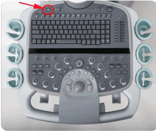
Fig. 8: S2000 Control Panel Power Button
