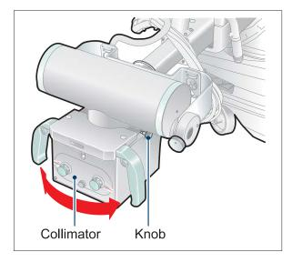
Rotate the X-ray tube unit laterally.
