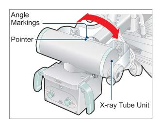
Coosen the knob, and rotate the X-ray tube unit forward and backward.
