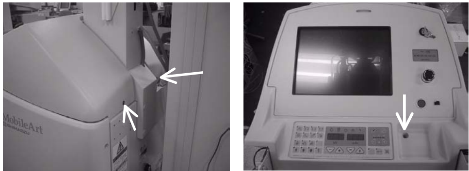
Fig. 6-4 Screw clamp positions of the top cover.
