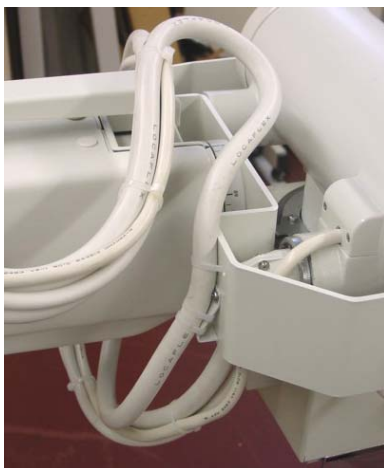
Fig. 6-33 Cable Treatment (Reference Drawing)
