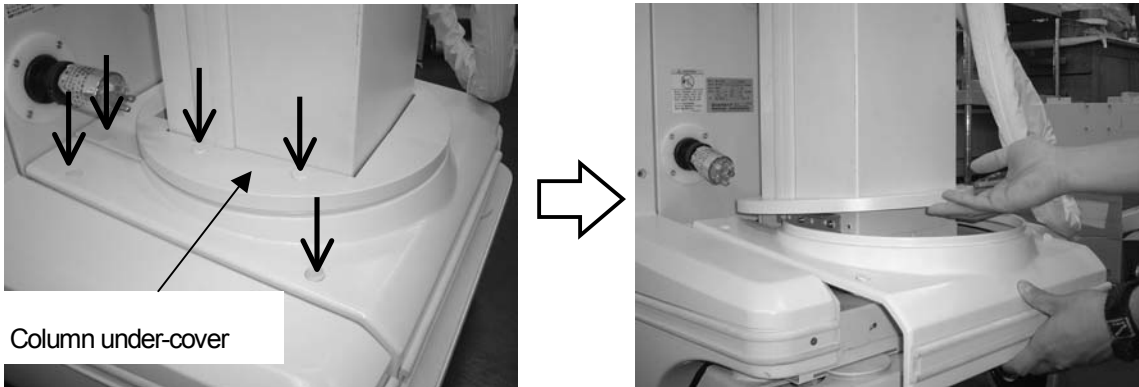
Fig. 6-6 Method of opening/closing the front side cover
