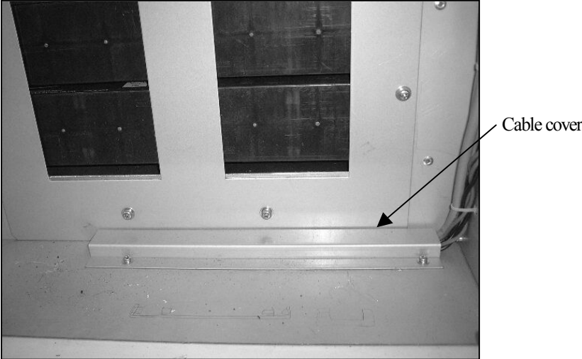
Fig. 6-53 Remove Cable Covers for DC motors
