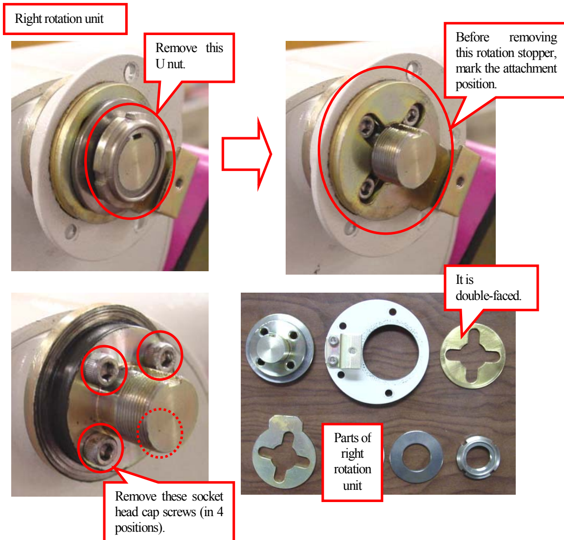
Fig. 6-28 Removing the Right Rotation Unit and Removed Parts
