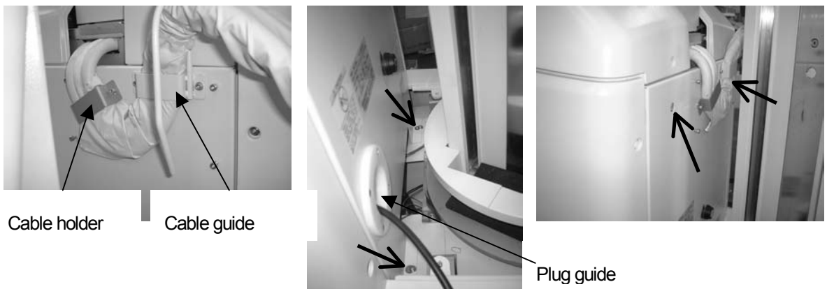
Fig. 6-9 Screw clamp positions of the front cover
