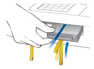
**6** Ensure that the battery is fully inserted into the slot. The pull tab will insert along with the battery. Insert the second battery following the same procedure.
