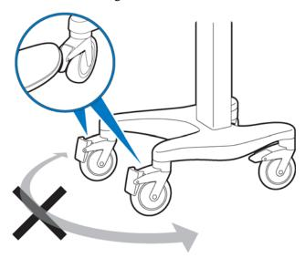
2 Step down on the gray rear wheel brake to lock the cart wheels. The cart will not move. Step on the wheel brake again to unlock the wheels.
