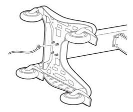
**4** Attach the bolt screws and tighten using the provided wrench. Ensure that the bolt screws are tightened to 80-100 in lbs.
