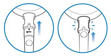
2 Connect the other end of the patient data cable to the PIM connector port ( ) located on the rear panel of the cardiograph. Align the raised circle on the cable connector upright as shown in the figure. Turn the cable connector to the right to lock it into position.
