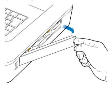
2 Locate the two gold pull tabs inside of the battery compartment. Pull the tabs straight out of the battery compartment and lay flat.
