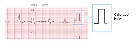
The shape of the calibration pulse reflects the scaling of the trace.
