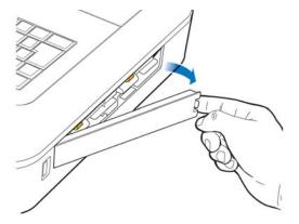
**4** Remove the batteries from the battery compartment by pulling on the gold straps.
