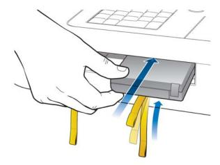
4 Push in the battery and ensure that the battery is fully inserted into the slot. The gold pull tab will insert along with the battery. Insert the second battery (if necessary) following the same procedure.
