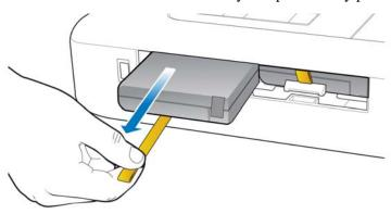
5 Insert the battery with the external connector facing the bottom rear of the compartment.
