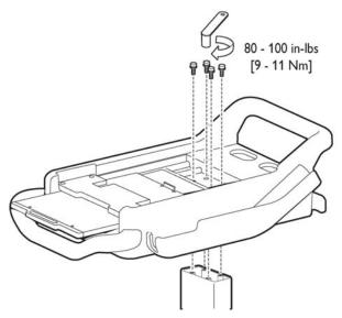
**10** Align the rear feet of the cardiograph with the rear holes on the cart. Lower the front feet of the cardiograph into the front holes on the cart and push the cardiograph into place. Ensure that the cardiograph is locked into the slot on the front right of the cart.
