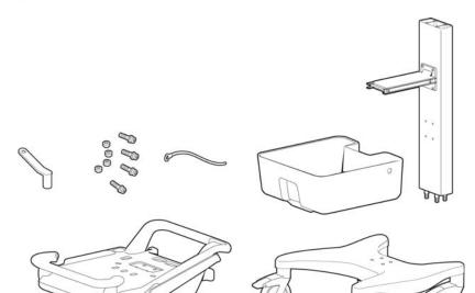
Figure 1-5 Unassembled Cart Kit Contents
