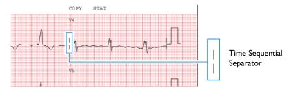
The single line indicates that the ECG data for each lead is displayed over a continuous period of time. For example, on a 3x4 grid all signals start at 0 in the first column, 2.5 seconds in the second column, 5.0 seconds in the third column, and 7.5 seconds in the fourth column.
