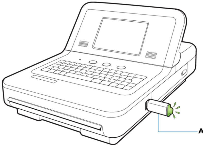
**A** USB memory stick inserted into USB connector (tip illuminates when properly inserted)
