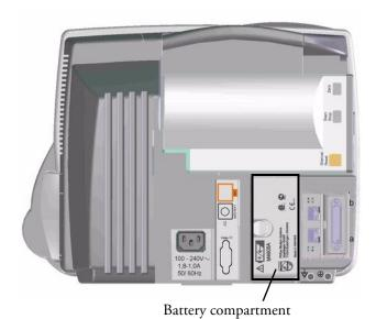
MP40/MP50: two Philips M4605A rechargeable Lithium Ion batteries must be inserted into the battery compartment at the rear of the monitor to use the MP40/MP50 monitor with battery power.
