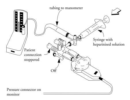
3 Move the syringe barrel in and raise the mercury to 200mmHg (30kPa). 200mmHg is the recommended calibration pressure.
