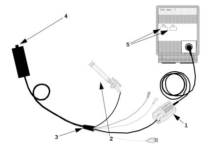
Connect the optical module (Hospira 50131) to the measurement module. Allow the optical module to warm up before you perform a calibration. Although the warm up message disappears from the screen after one minute, Hospira recommends letting the optical module warm up for 15 minutes for best accuracy. Please refer to the instructions for the optical module.
