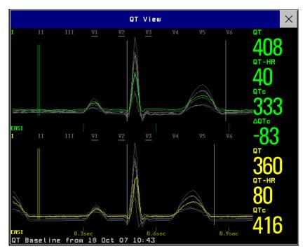
The current waves are shown in the upper half of the window and the baseline waves in a different color below. The Q and T points are marked with a vertical line. By selecting one of the lead labels at the top of the window you can highlight the corresponding wave; the other waves are shown in gray. The underlined lead labels are the leads used for the QT calculation. By selecting the numeric area you can highlight all underlined leads.
