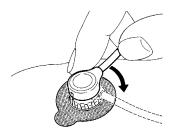
3 Apply the transducer as soon as possible after you see the "...calibration complete" message. If you wait longer than 30 minutes, the heat supply to the transducer switches off to prevent the electrolyte from drying out and a new calibration is necessary.
