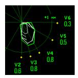
In this diagram, V4 was either temporarily switched off, or in INOP, for around 30 seconds. No data was recorded. Consequently, the affected maps are not closed.
