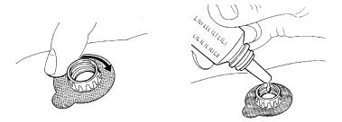
2 Align the arrow on the transducer with the tab on the ring and fasten by turning turn a quarterturn clockwise. Wait 10-20 minutes for readings to stabilize.
