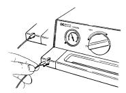
2 Plug the transducer cable into the module. Swing the calibration chamber cover open and insert the transducer into the chamber. Close the cover to secure the transducer. Set the transducer temperature at the monitor now.
