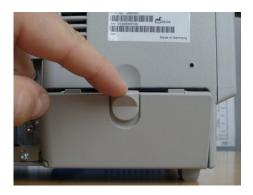
MP40/MP50 You can replace batteries without switching off the monitor, if you replace them one at a time and if the remaining battery has sufficient power. The **Battery MISSING** INOP is suppressed for 30 seconds while you exchange each battery.
