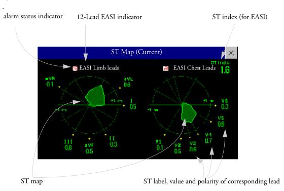
If an ST lead is switched off, its axis is not shown in the map.
