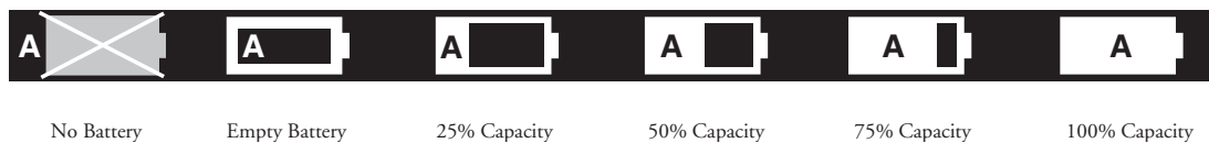
Figure 6 Battery Charge Level Indicators
