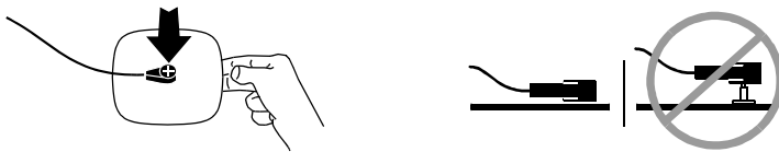
Figure 5-4 Connecting FAST-PATCH Electrodes to Defibrillation Cable
