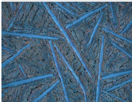
Hypereutectic white pig iron, primary cemented plates, 100 x polarized light, with various Lambda settings
