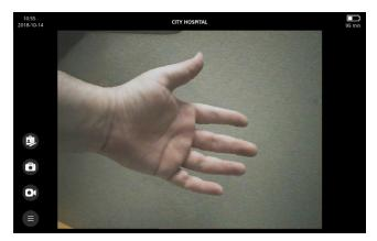
Note: There may be a slight blade intrusion in the upper-left corner of the monitor, and a thin line may appear along the top. These blade edges are captured in the view because of the wide-angle camera lens used in the video laryngoscope. This image acts as a frame of reference during the intubation process and ensures that the orientation of the image is correct in the monitor.
