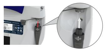
3. To disconnect the video cable from the monitor, rotate the connector ring in the direction of the release arrow, and then remove the connector from the port.
