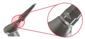
2. To disconnect the scope from the video cable, hold the scope in one hand, twist the cable's locking collar in the direction specified by the arrow on the collar, and then pull. The scope disconnects from the cable.
