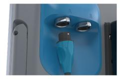
2. To disconnect the video cable, hold the cable connector in one hand and support the monitor with the other, and then pull. The cable disconnects from the monitor.
