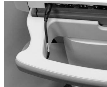
Not enough cable slack.
