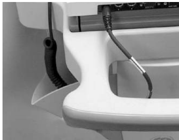
Correct amount of cable slack.
