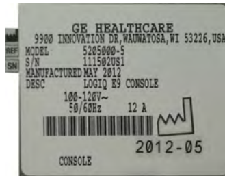
Figure 4-5. Rating Plate–USA/Asia 120V console
