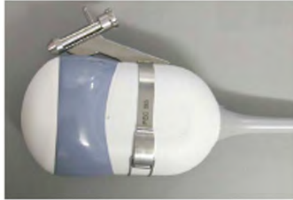
Figure 1-42. Mounting the Biopsy Needle Guide to the 4D Probe
