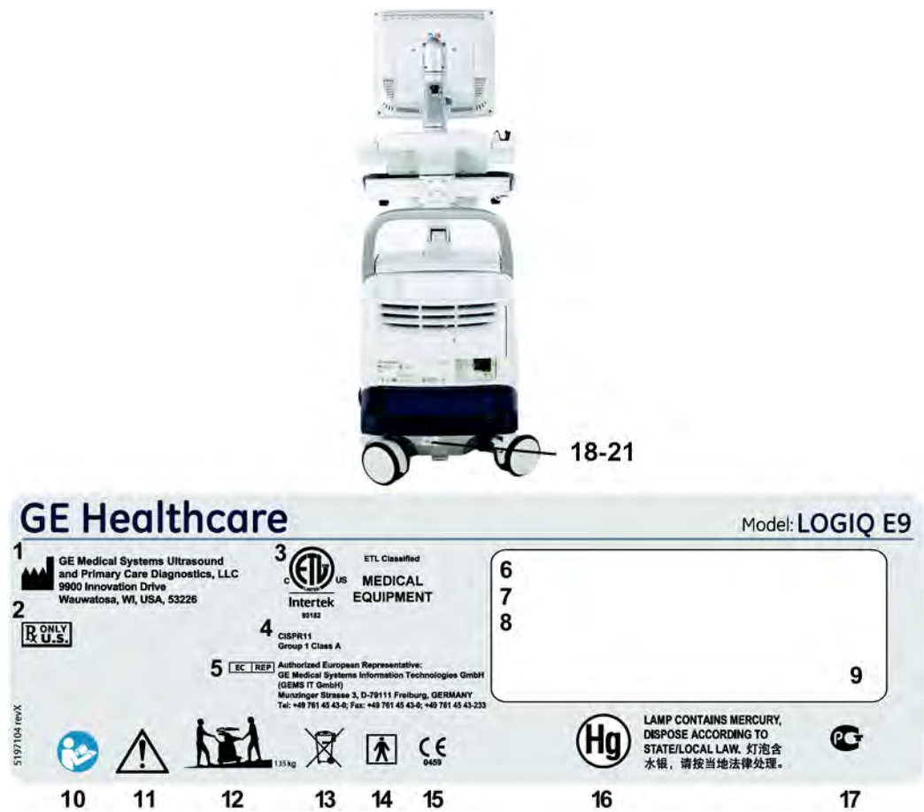
Figure 4-2. Rear Panel Label Location
