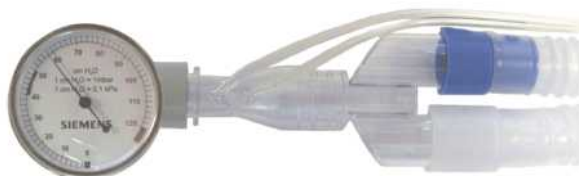
Manometer Reading 58 cmH2O
