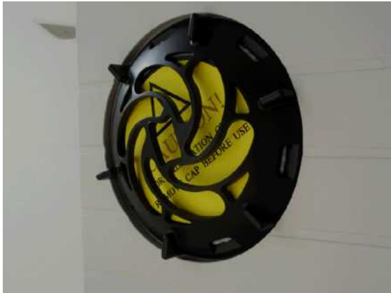
Figure 7-8 O2 Calibration Cover
