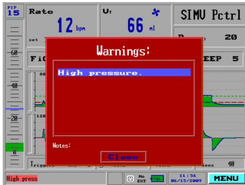
Figure 8-5 High Pressure Alarm
