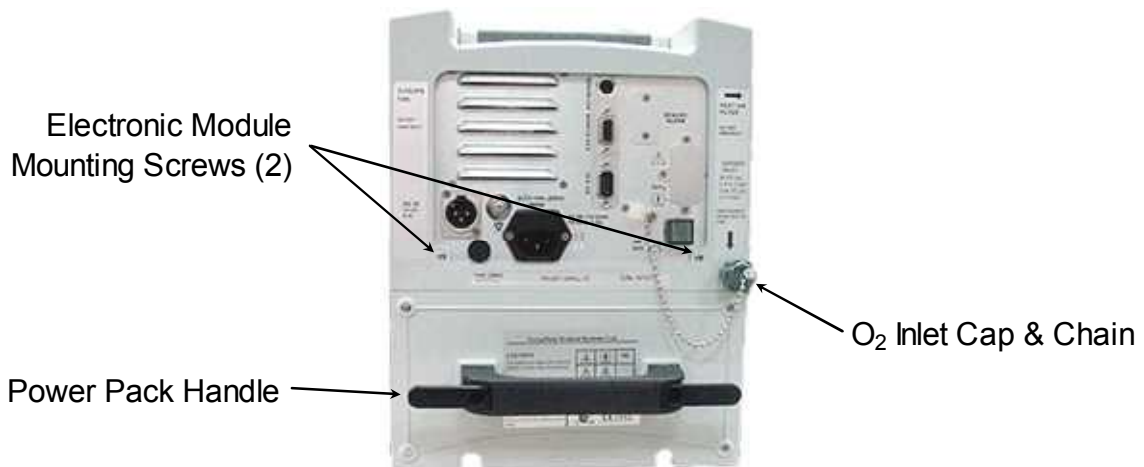
Figure 11-4 Enclosure (Rear View) #2
