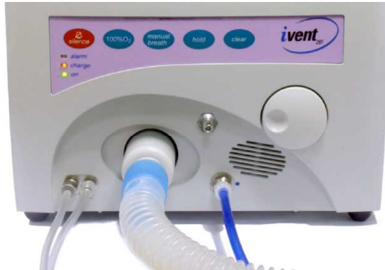
Figure 3-4 Patient Circuit Connection
