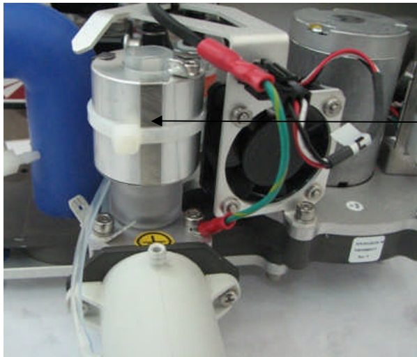
Figure 11-11 The O 2 sensor location on the pneumatic unit
