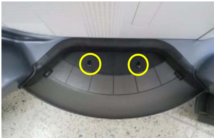
Figure 8-20 Unscrewing 2 screws and remove SIDE TRAY ASSY
