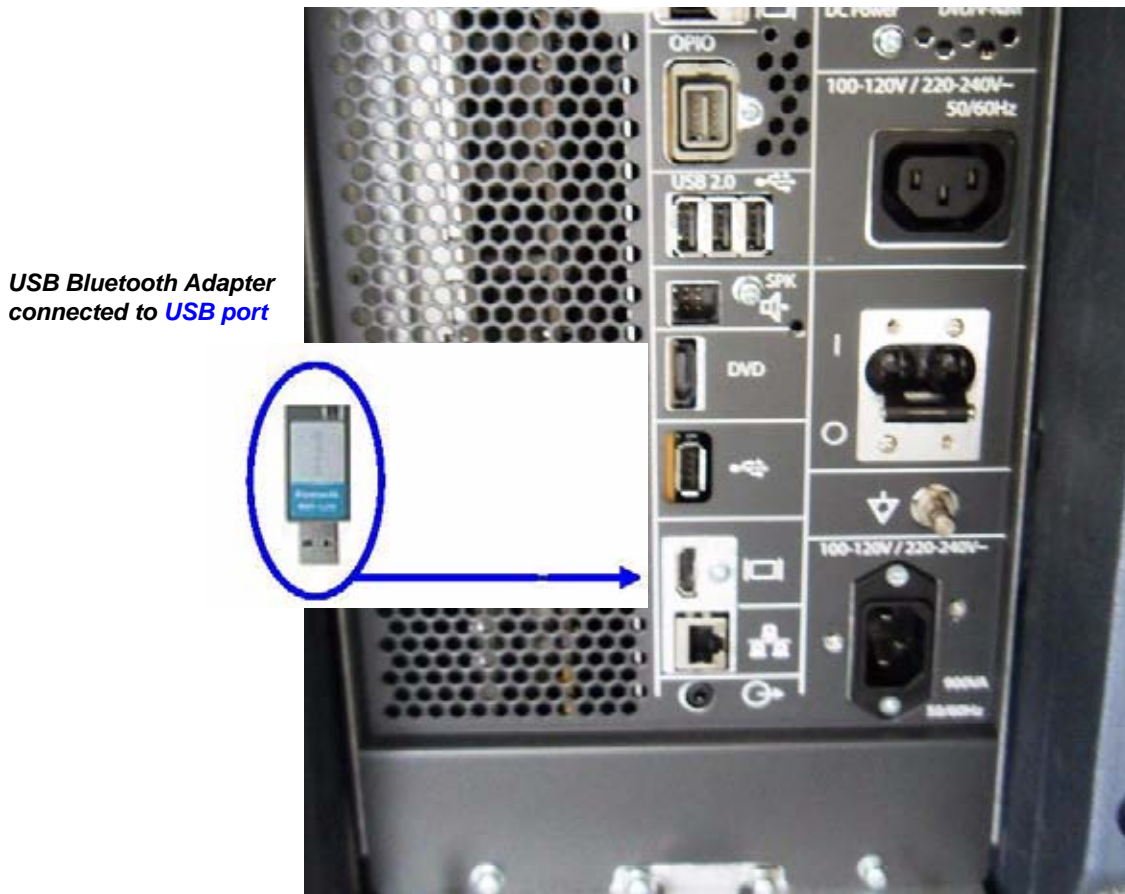
Figure 3-8 HP Officejet H470 DeskJet Printer connection (via Bluetooth Adapter)
