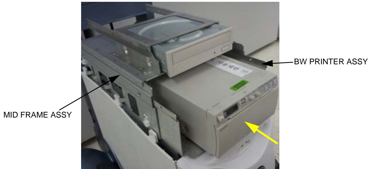
Figure 8-26 Insert BW PRINTER ASSY to MID FRAME ASSY
