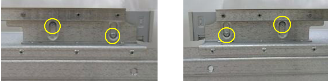
Figure 8-56 Unscrew 4 screws to remove the DVD (Left / Right)
