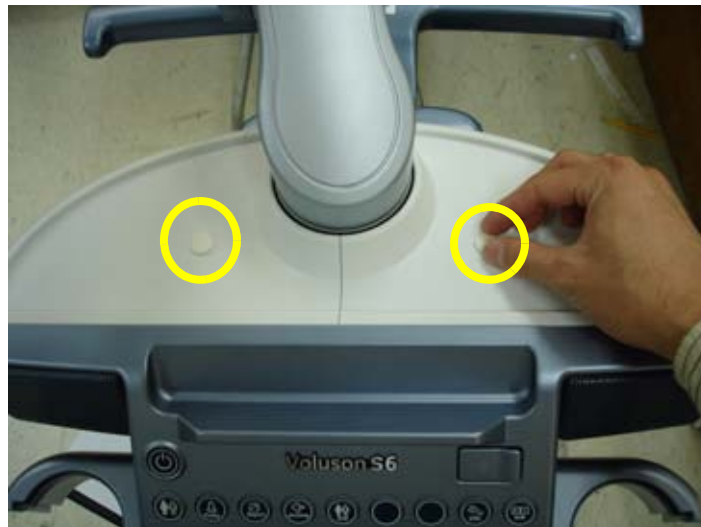
Figure 8-21 Removing the RUBBER CAP
