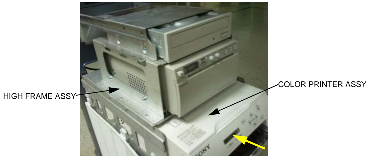
Figure 8-45 Insert COLOR PRINTER ASSY to HIGH FRAME ASSY
