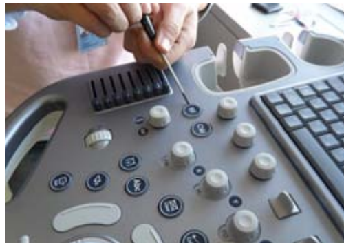
Figure 8-23 Push against the circle cap and lift it
