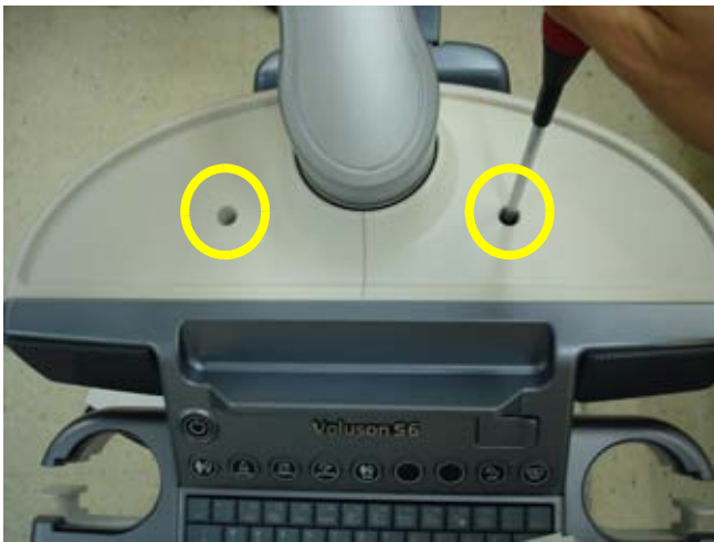
Figure 8-22 Removing the OPIO COVER L, R
