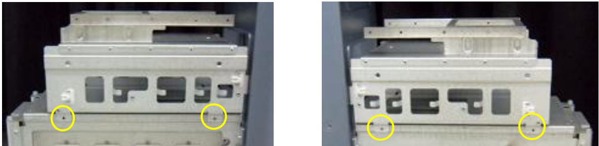
Figure 8-58 Unscrew 4 screws and remove MID FRAME ASSY
