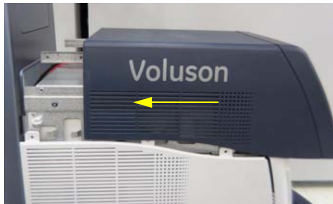
Figure 8-79 Place MID CABINET on MID FRAME and Moving toward BACKBONE
