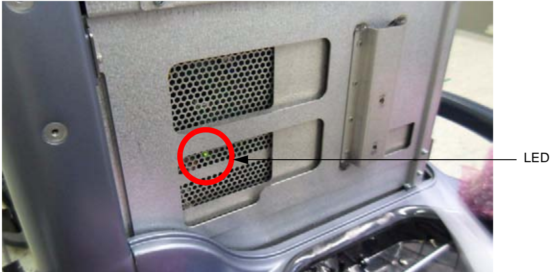
Figure 7-6 Check green LED inside CPS
