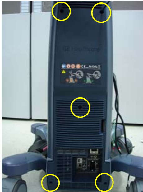
Figure 8-59 Unscrew 5 screws and remove REAR COVER POLARIS ASSY
