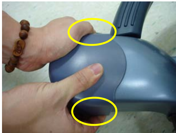
Figure 8-15 Removeing the CASTER CAP
