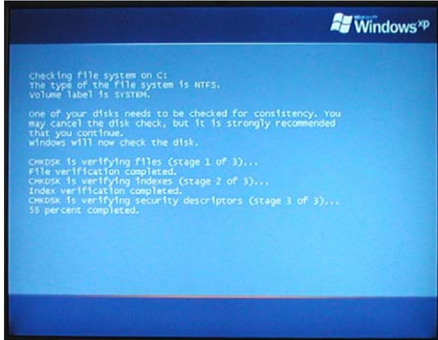
Figure 8-8 Check disk is performed automatically
