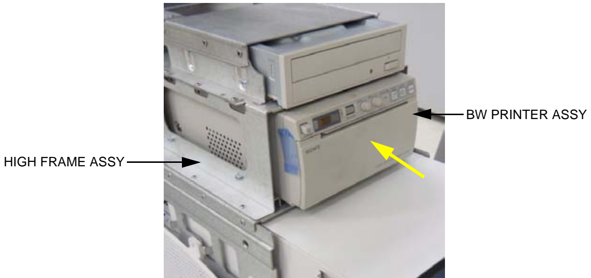
Figure 8-36 Insert BW PRINTER ASSY to HIGH FRAME ASSY
