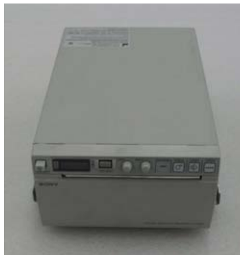
Figure 8-35 Fix BW PRINTER to BW BRKT POLARIS with 4 screws (2306562, FH M3X6)
