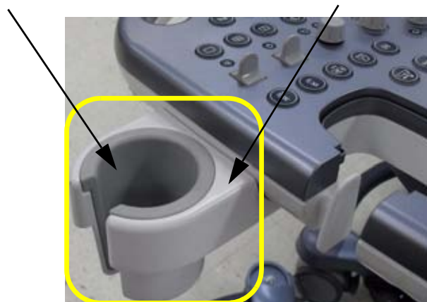
Figure 8-85 Insert TV PROBE HOLDER RUBBER to PROBE HOLDER BASE
