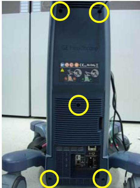
Figure 8-28 Unscrew 5 screws and remove REAR COVER POLARIS ASSY
