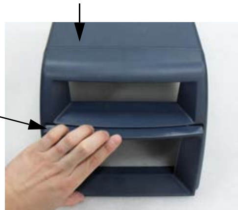
Figure 8-32 Assemble DUMMY CASE MID BW POLARIS with MID CABINET ASSY
