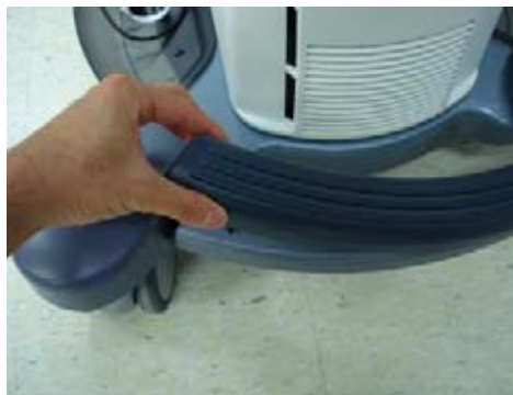
Figure 8-19 Removing FOOTREST COVER
