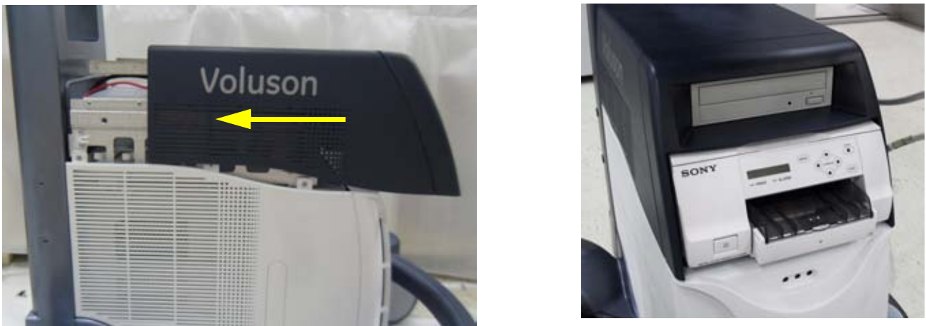
Figure 8-43 Assemble MID CABINET ASSY
