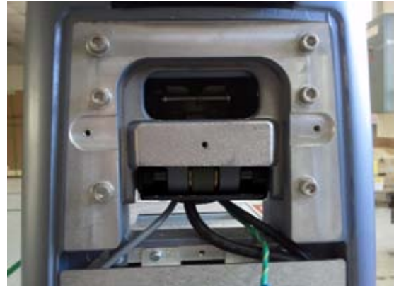
Figure 8-73 ELEVATION ARM DOWN STOPPER HIGH POLARIS with 2 Hexagonal screws (5405682, HSH M6x30)
