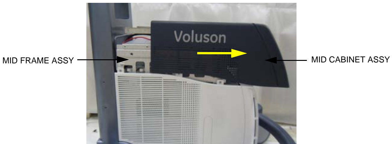
Figure 8-24 Moving forward MID CABINET ASSY following Slide Rail
