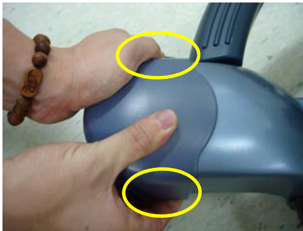
Figure 8-16 Removeing the CASTER CAP
