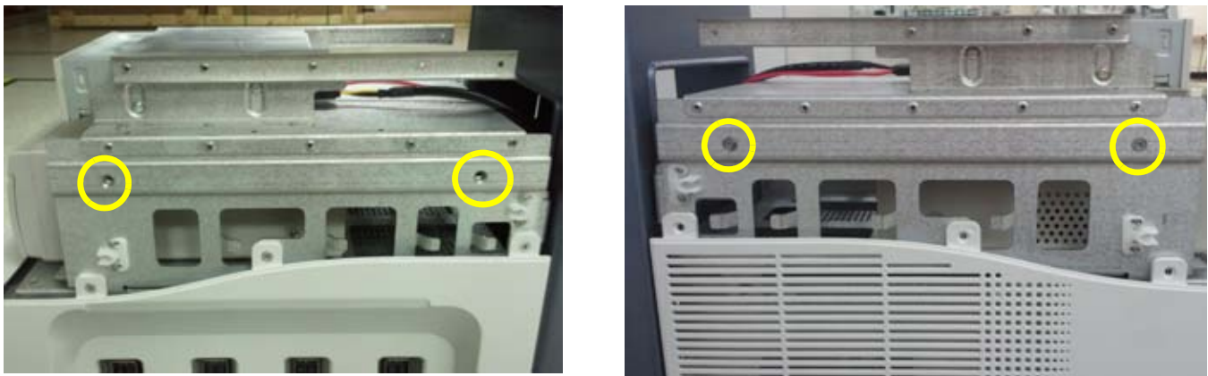
Figure 8-27 Assemble BW PRINTER ASSY to MID FRAME ASSY with 4 screws (5178673, SCREW FH M4X6)
