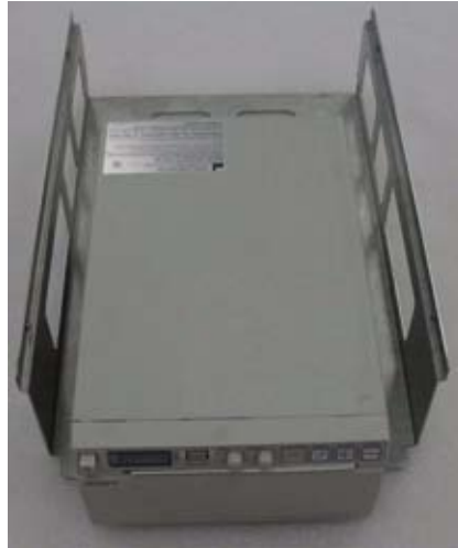
Figure 8-25 Fix BW PRINTER to COLOR PRINTER BRKT POLARIS with 4 screws (2306562, FH M3X6)
