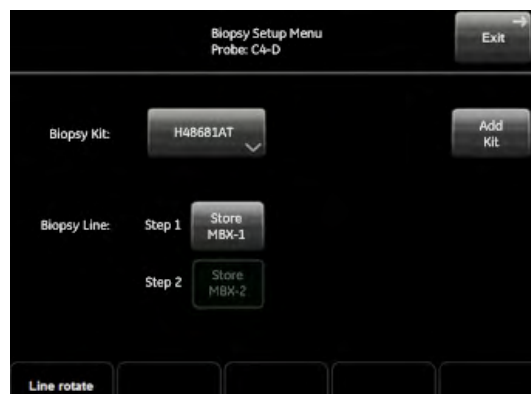
Figure 5-2 Biopsy Setup Menu: Multi angle biopsy guide
