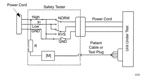
For the protection of the test person, the following values of resistor R may be used.
