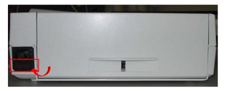
6. Position plastic fuse tray and snap back into position.
