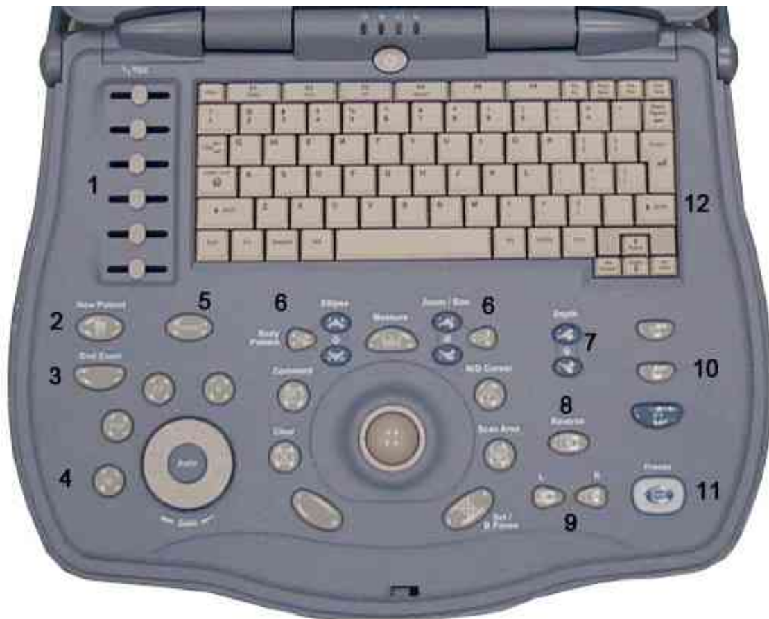
Figure 4-6 Control Panel Tour
