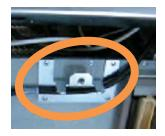
Make sure the GFI PCIe cable is routed behind the MPS fang as shown on the left. This is for the GFI Configuration only. MRX systems do not have this cable.
