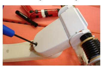
Remove the 16 screws securing the second arm section cover with Philips screwdriver.
