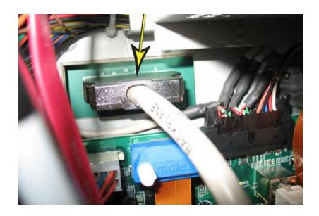
Or, the Backplane cable, J3 (right) and J5 PCIe to the Card Rack on a GFI Configuration, using a BEP6 as shown below. Keep the cable to transfer to the replacement BEP.
