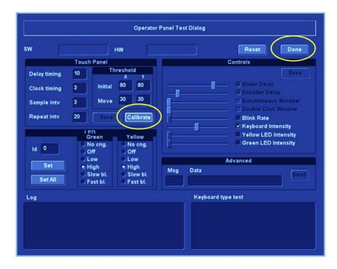
The **Calibrate** button is used to start to calibrate the position of the touch sensitive area on the touch screen relative to the graphic artwork.
