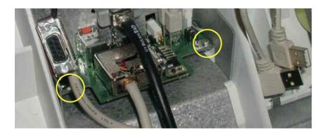
Unscrew and remove the two screws and remove the Bulkhead Board.
