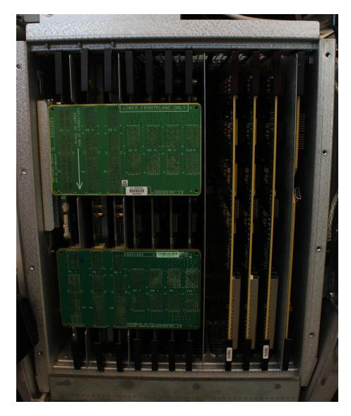
Repeat those steps until the two XD\_Bus boards release from remaining FEP boards.
