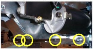
Remove these four screws the Z mechanism:
