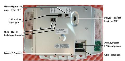
Next disconnect the cables as shown below at the back of the Upper OP Panel/Touch Panel Assembly.
