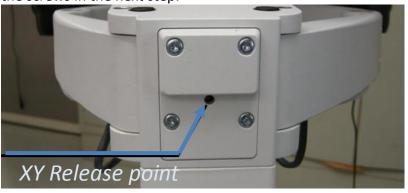
Use thumbs to press upper lock tabs toward the front of the system to release the top of the Bulkhead Cover.
