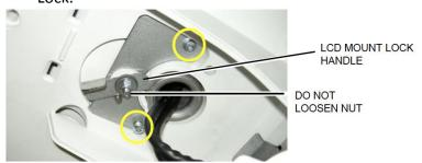
LCD Mount Lock reinstallation procedure:
