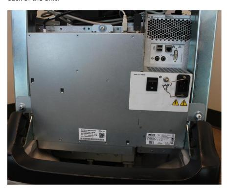
Power from the wall outlet (100 to 240 VAC, 50/60 Hz) is connected to the Main Power Supply. The MPS delivers the needed voltages to the rest of the Logiq E9/Vivid E9:
