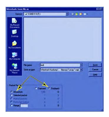
This saves the DICOM traffic in a file with suffix ".pcap", which can be analyzed by Wireshark or a similar network sniffer.
