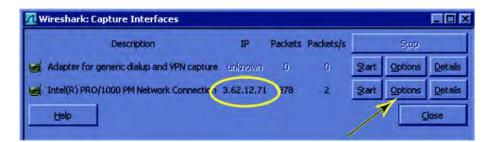
In the Capture/Interfaces window press the Options button that corresponds to the IP address.
