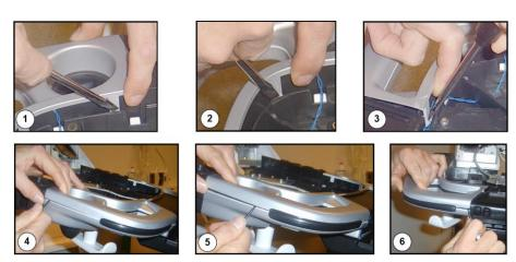
Use a thin screwdriver to release the hatches, one by one as illustrated, until you can remove the handle.
