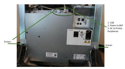
Disconnect the cables from the top of the power supply.
