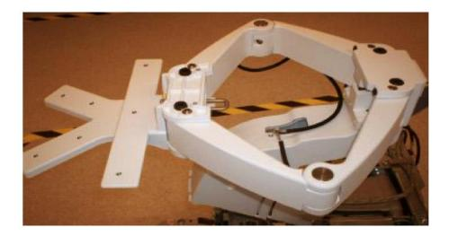
Remove the four screws for the XY (Frogleg) mechanism and remove the XY mechanism.
