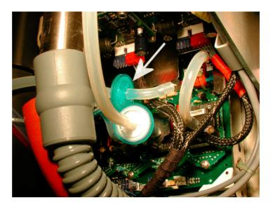
Figure 13 Sampling-gas return-line filter
