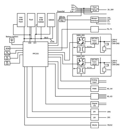
Figure 4 Block diagram of the VERONA PCB
