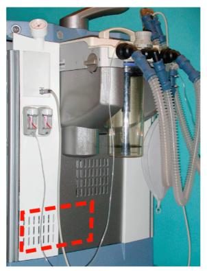
Figure 4 Fitting location of the power supply unit in the Zeus
