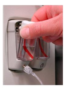
Figure 1 Removing the water trap
