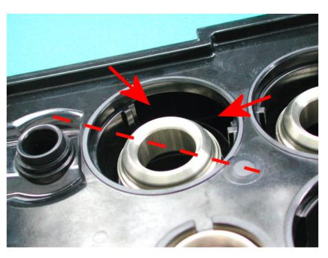
Figure 10 Diaphragm mount location hole
