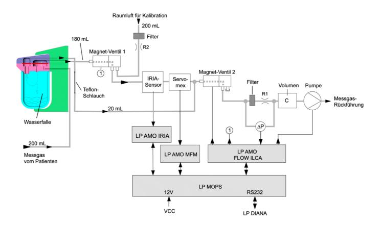
Figure 20 PGA block diagram (example GMZ)
