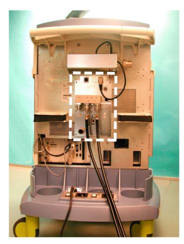
Figure 17 CS module fitting location
