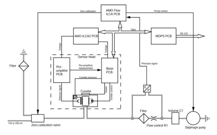
A pneumatic low pass, comprising the volume C1 and the flow control valve R1, minimises the pressure surges generated by the pump (Figure 32).
