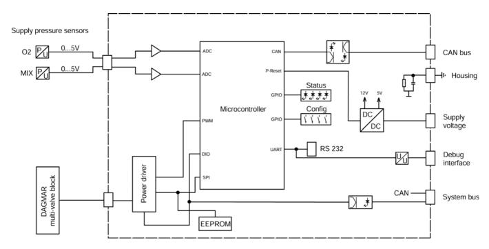
Figure 12 Block diagram of the DAGMAR PCB
