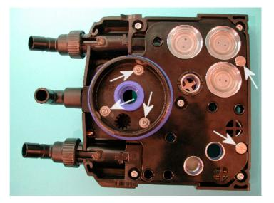
Figure 8 Plate fixing screws
