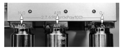
Figure 16 NIST and cylinder connection markings
