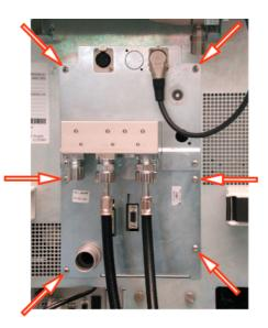
Figure 18 CS module fixing screws
