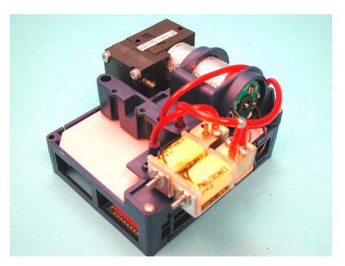
Figure 21 IRIA module without sensor
