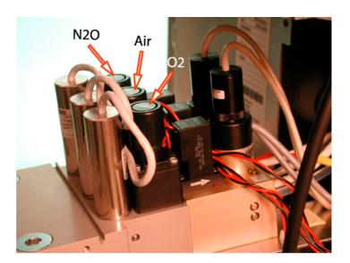
Figure 22 Assignment of pressure regulators
