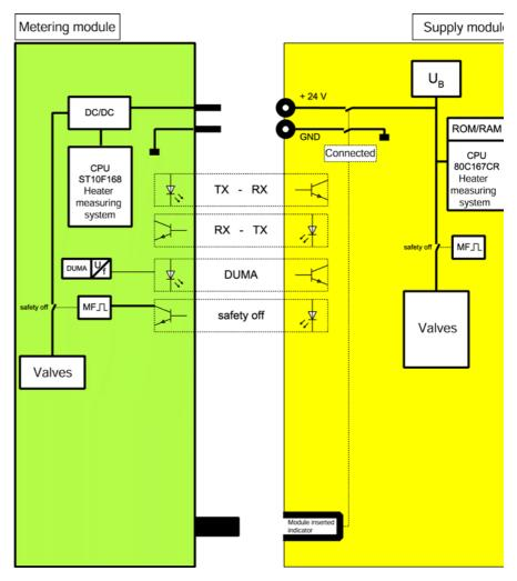
Figure 14 Optical and electrical interfaces
