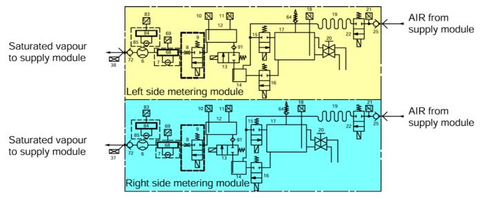
Figure 17 Metering module gas flow diagram
