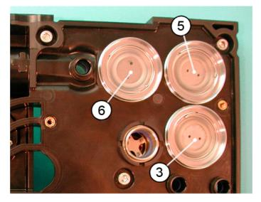
Figure 9 Flow (6), Spont (5), and Closed valve (3), old version
