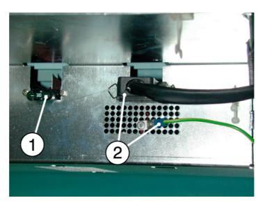
Figure 24 Fuse (1) and connector (2) on drawer unit
