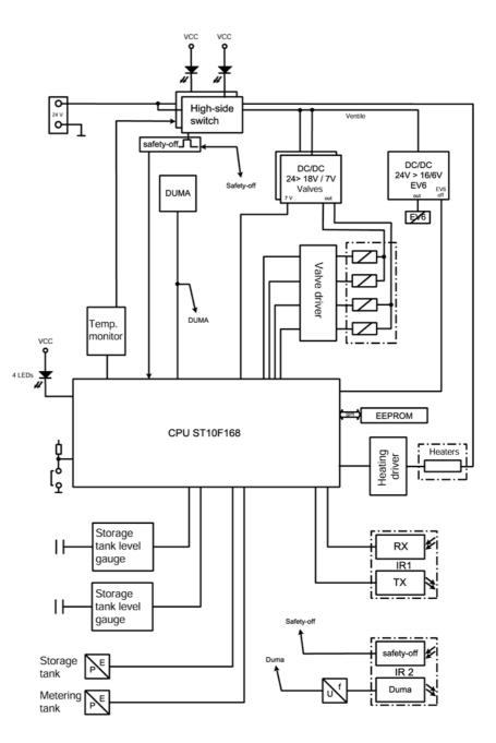
Figure 18 Block diagram of the Metering Module PCB
