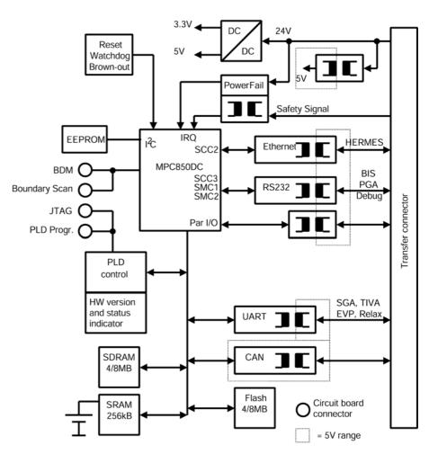
Figure 3 Block diagram of the DIANA PCB
