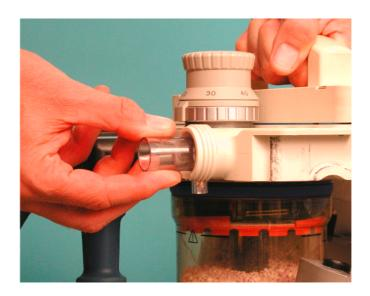
Figure 12 Removing the flow sensor
