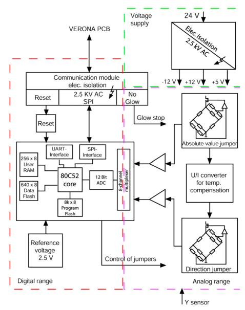
Figure 6 External Flow PCB block diagram
