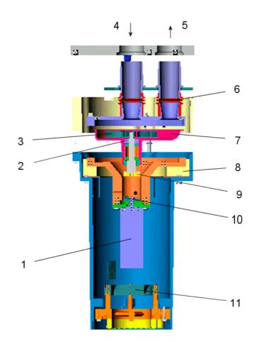
Figure 38 Blower sectional diagram
