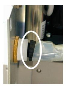
Figure 19 Power switch with lock nut
