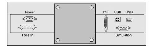
Figure 43 Monitor connections
