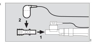
3 Plug the CO2-sensor connector into the »CO2 🔊 « socket on the rear of the device.
