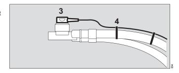
5 Insert the connector for the temperature-sensor into the **»Temp** ★ « socket at the rear of the unit.
