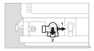
If the expiration valve is fitted with an optional water trap:
