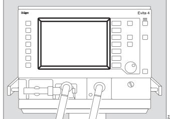
The keys for routine functions are placed to the right and left on the outside of the front panel.
