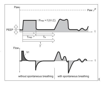
This effect can also be caused during ventilation, e. g. due to a build-up of secretion. In this situation, the pressure is limited by the alarm limit »Paw \_/\*« The pressure rise stops 5 mbar below the alarm limit »Paw \_/\*« and the alarm
