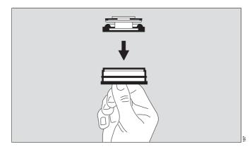
Insert stopper with diaphragm assembly on top into the housing from below and screw in tightly.
