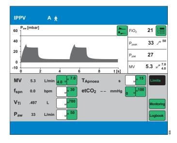
1 Touch the relevant screen key for the alarm limits, e. g.: MV 2.3 L/min » [3.1] (\*\*)
