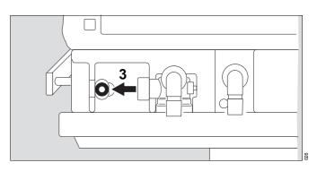
4 Fit flow sensor – with the connector facing towards the ventilator – into the mounting and push into the socket as far as it will go.
