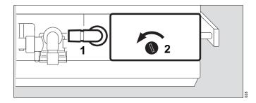
3 Loosen the two knurled screws and open the sensor housing.
