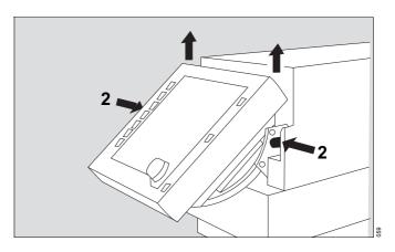
3 Lock it into position = pull tab under the holder down and turn it towards the wall rail.
