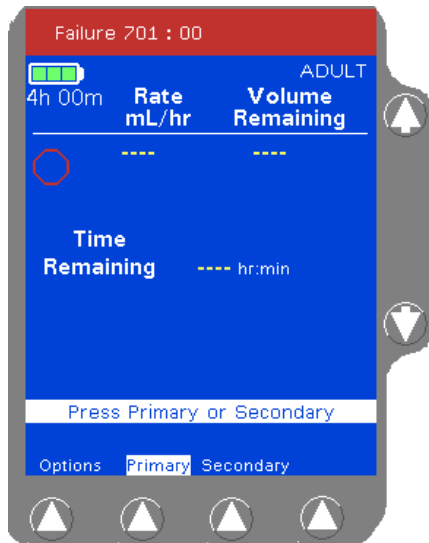
Figure 8-2 Channel Failure Status Line Display
