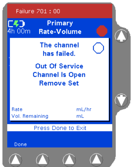
Figure 8-3 Channel Failure Pop-up Message
