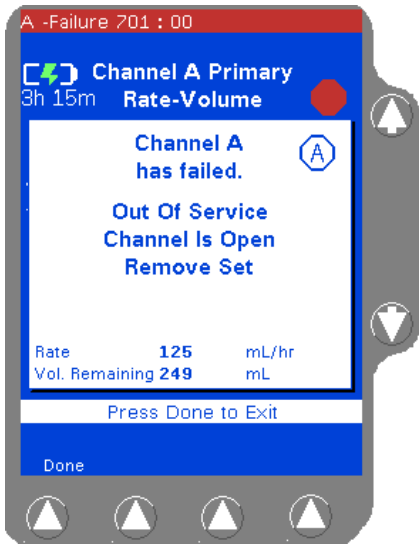
Figure 8-6 Channel Failure Pop-up Message
