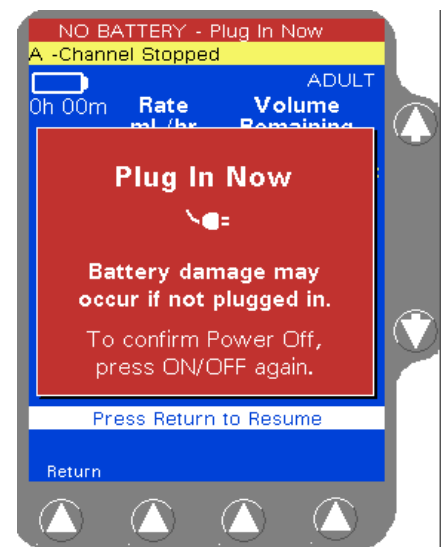
Power Off Pop-up on Depleted Battery
