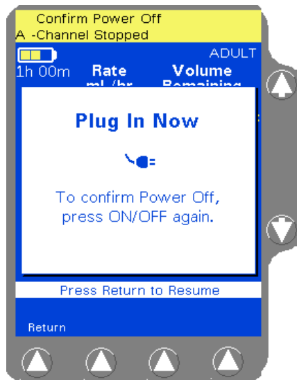
Power Off Pop-up on Battery Power
