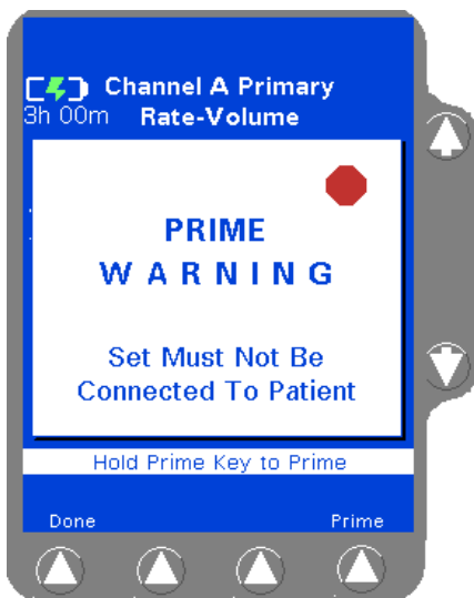
Figure 4-22 Ready to Prime
