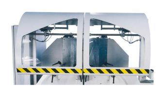
Minimum cutting length between 2 blades 370 mm
