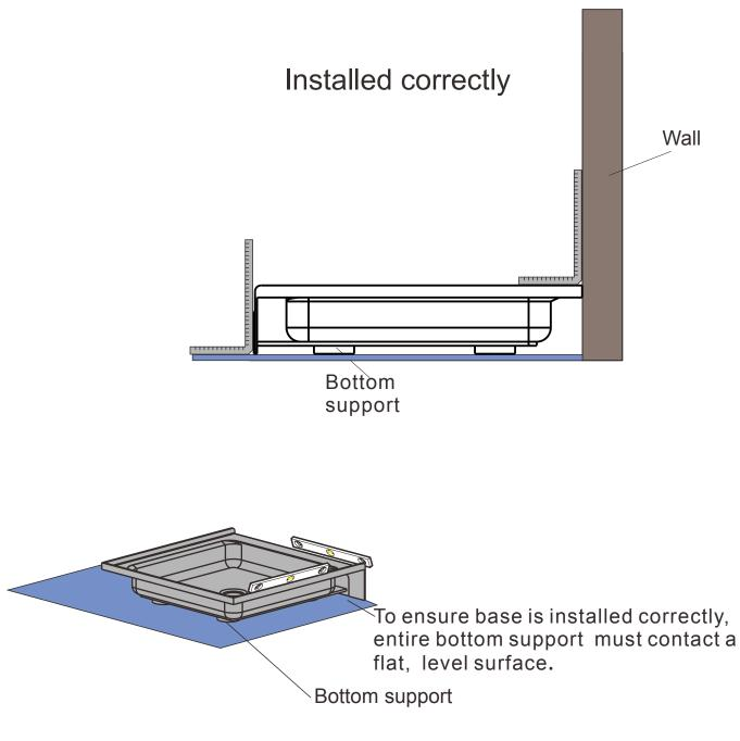
Do not install the product with any air gaps under the bottom support or product damage will occur.
