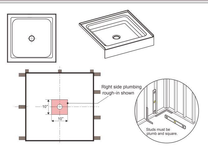
\*Rough plumbing must be installed before bathtub installation.
