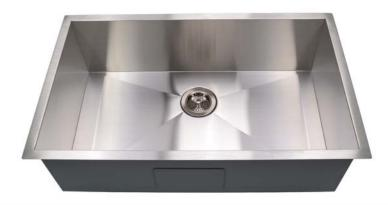
**18 GAUGE BRUSHED FINISH SINGLE BOWL FULLY INSULATED SPRAY & PADS** SCORED DRAINLINES **ZERO CORNER RADIUS REAR SET DRAIN CLIPS & TEMPLATE INCLUDED** OUTSIDE DIMENSION: 32"L X 19"W INSIDE DIMENSION: 30"L X 17"W **DEPTH: 10" INSTALLATION : UNDERMOUNT** DRAIN: 3 1/2" **CONFIGURATION: SINGLE BOWL MINIMUM CABINET SIZE: 34"**
