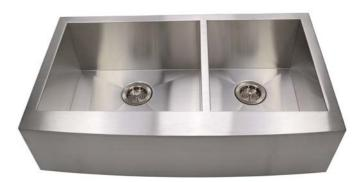
16 GAUGE BRUSHED FINISH DOUBLE OFFSET BOW/ CURVED APRON FRONT FULLY INSULATED SPRAY & PADS SCORED DRAINLINES ZERO CORNER RADIUS REAR SET DRAINS CLIPS & TEMPLATE INCLUDED OUTSIDE DIMENSION: 35 3/4" L X 20 3/4 W INSIDE DIMENSION: 33" L X 16" W DEPTH: 10" INSTALLATION : TOPMOUNT, UNDERMO INSET DRAIN: 3 1/2" CONFIGURATION: DOUBLE BOWL
