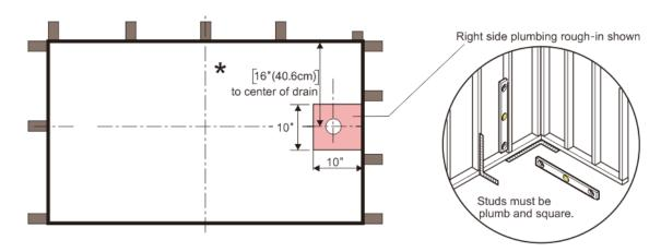
\* Rough plumbing must be installed before bathtub installation.
