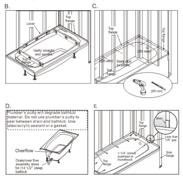
TIP: Place drop cloth in bathtub and stand inside bathtub to press it to floor when securing to wall studs.
