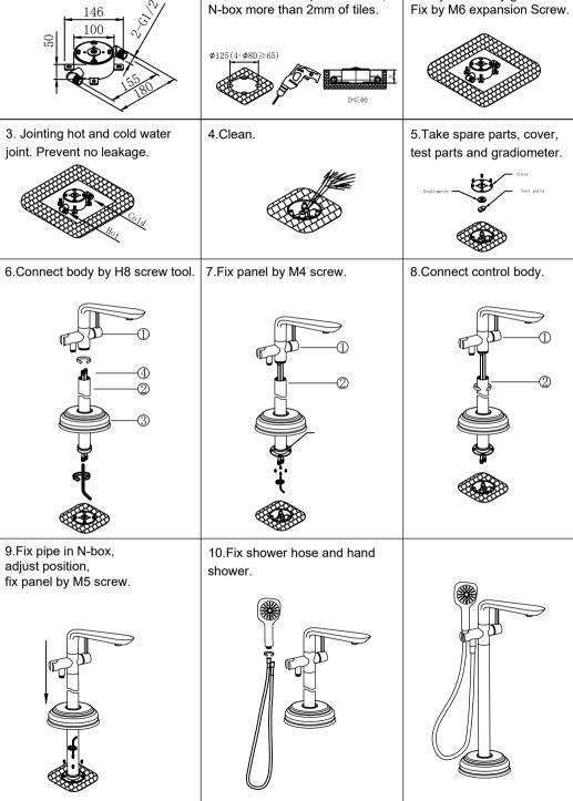
1.N-box in-wall depth:D≤46mm,
