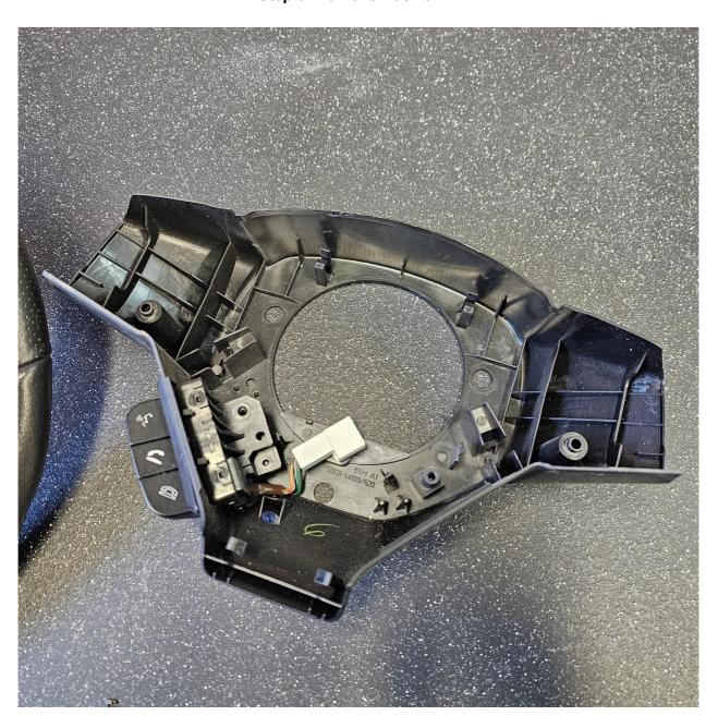
Step 6. Release button pack clips to release button pack from steering.
