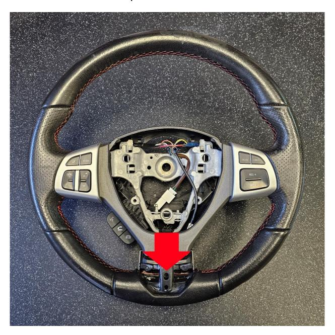
Step 4. Release 2 clips marked with red arrow (green arrow showing direction).
