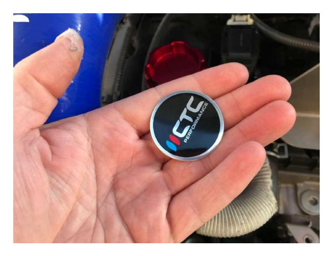
3. Turn over the logo plate, you will see double sided tape. Peel back the top layer leaving the adhesive on the oil cap.
