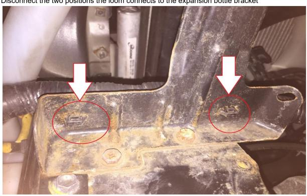
**Step 11**Undo 2 x 10mm bolts securing the expansion bottle bracket to the car and remove the bracket
