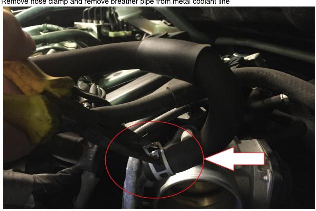
**Step 17**Remove clamp and hose from thermostat housing. You may lose a small amount of coolant which will need to be replaced
