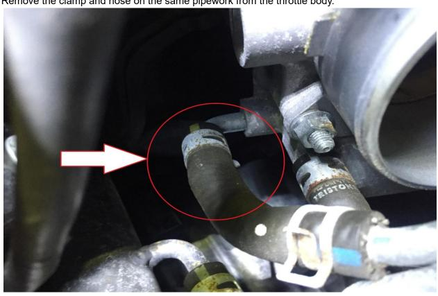
**Step 19**Replace this pipe with new silicone coolant hose supplied and 2 x jubilee clips supplied
