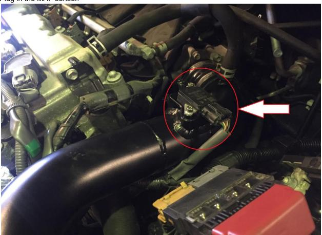
**Step 33**Secure the cables together using cable tie as pictured
