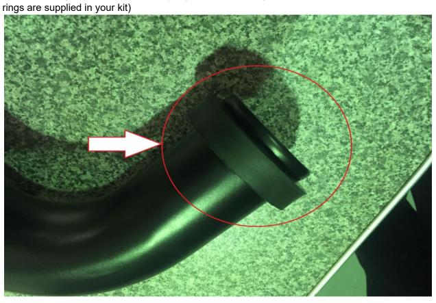
**Step 26**Press the filter over the intake pipe. Secure the filter using the jubilee clip supplied.
