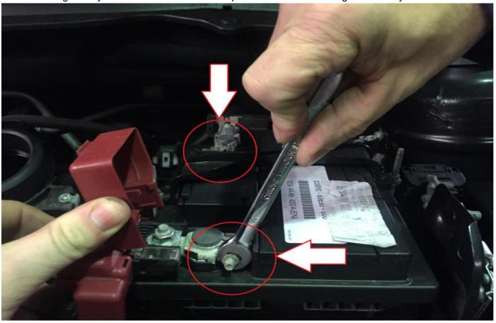
**Step 6**Undo 2 x 8mm nuts and remove battery clamp. Remove the battery and plastic tray below battery
