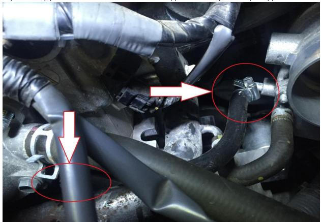
**Step 20**Remove 12mm nut to remove bracket remembering to replace the nut once bracket is removed.
