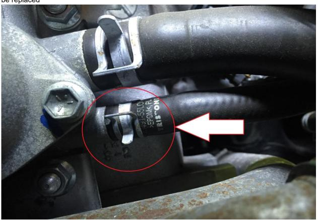
**Step 18**Remove the clamp and hose on the same pipework from the throttle body.
