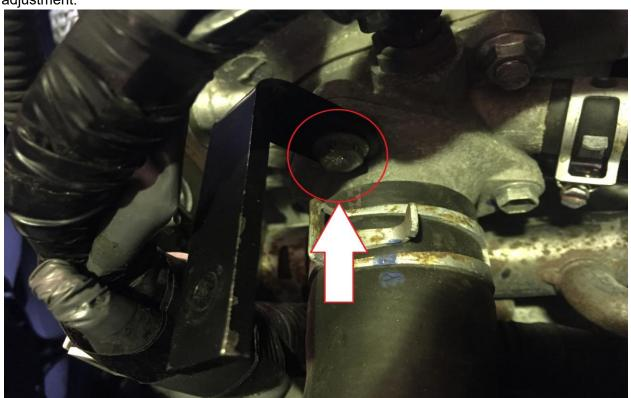
**Step 29**Fit intake pipe into position and secure to 90 deg bracket using M6 x20 bolt and nut supplied.
