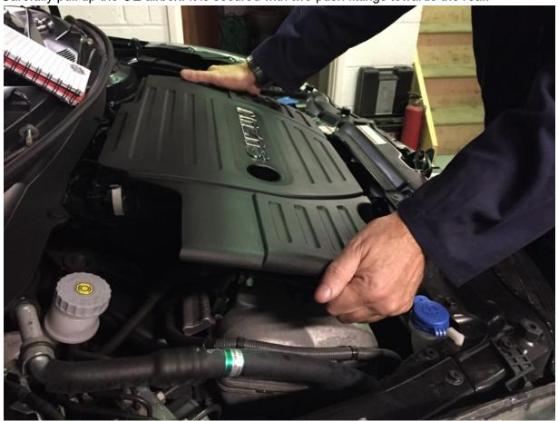
**Step 4**Remove 1 x bolt using a 10mm socket. Remove rubber intake pipe and plastic res. Remove Expansion Bottle from radiator.
