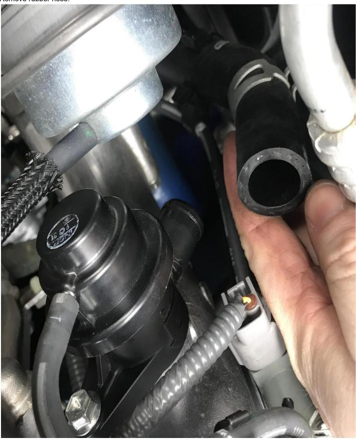
**Step.3**Remove Spring Clamp from Lower Vaccum Line from the solenoid.
