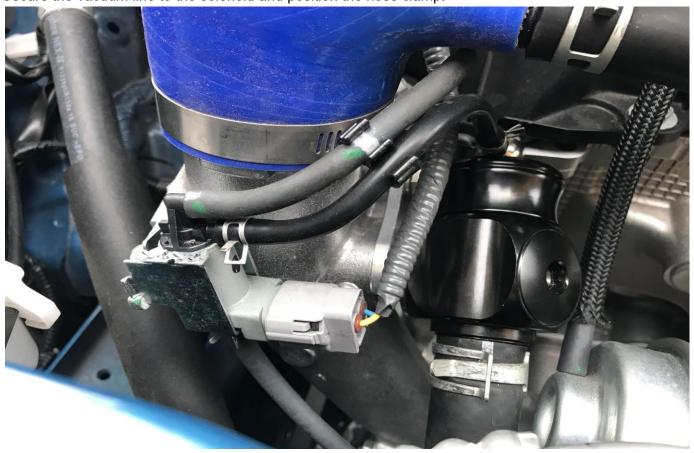
If you wish to run as Recirculation only fit as pictured above, if you wish to vent 50% of the air to Atmosphere for the most sound using a allen key remove the blank and screw in the trumpet provided as pictured below.
