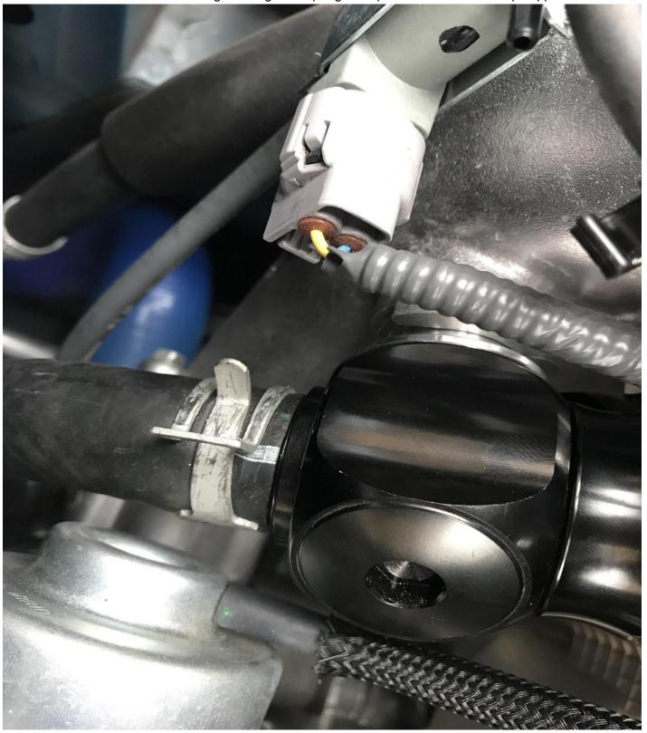
Now position the vacuum line and trim to length using scissors.
