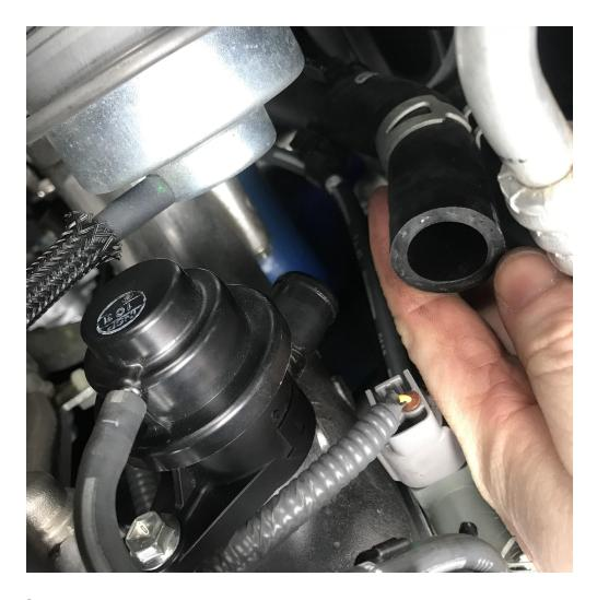
**Step.3**Remove Spring Clamp from Lower Vaccum Line from the solenoid.
