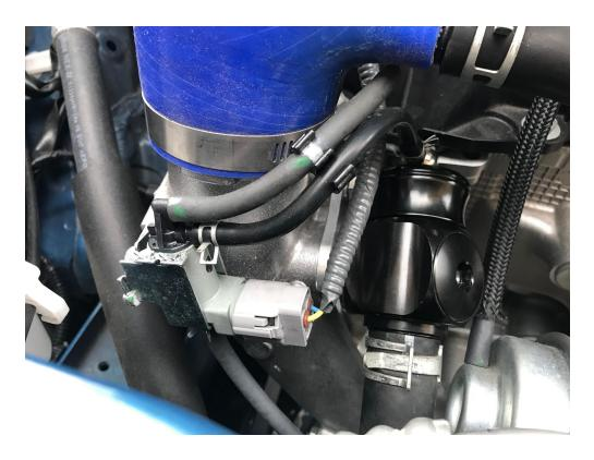
If you wish to run as Recirculation only fit as pictured above, if you wish to vent 50% of the air to Atmosphere for the most sound using a allen key remove the blank and screw in the trumpet provided as pictured below.
