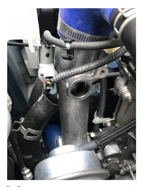
**Stage 7.**Fit one of the two OEM spring clips onto the new vaccum line as pictured.
