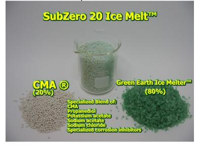
A 20% CMA, and 80% corrosion resistant chloride blend was shown to provide a 70-80% reduction in corrosion. SubZero 20 is a special blend that is even more effective in corrosion prevention, and at a lower cost.
