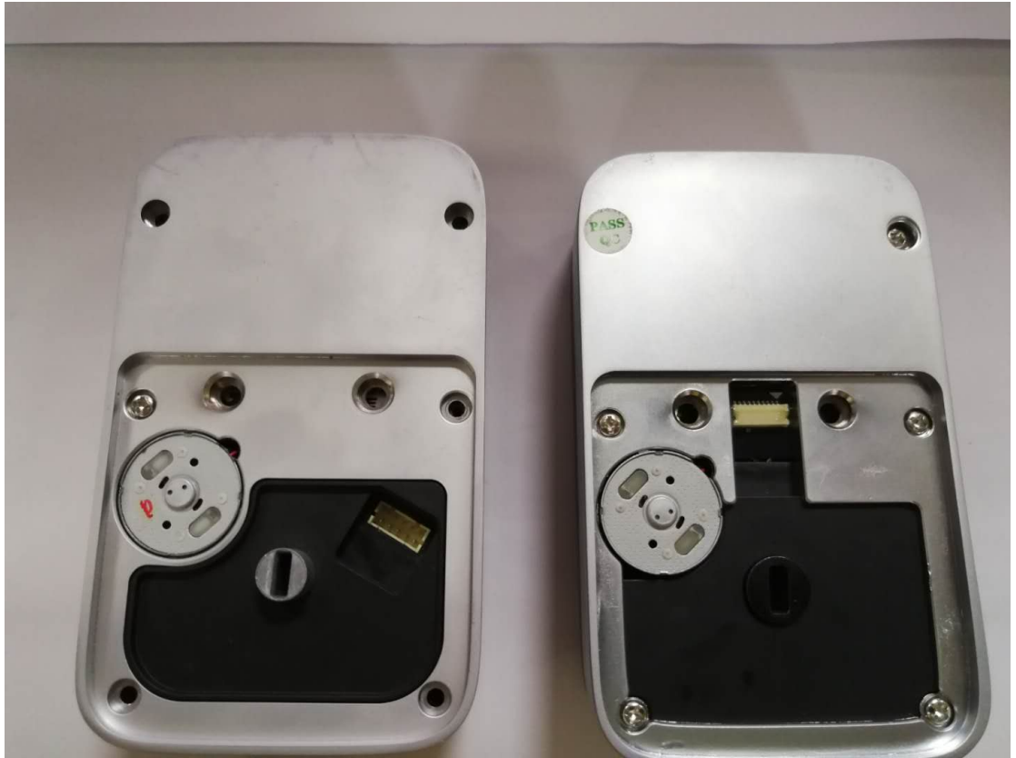
Easier to plug in cable. Stronger interface on PCB, which can hold more firmly.
