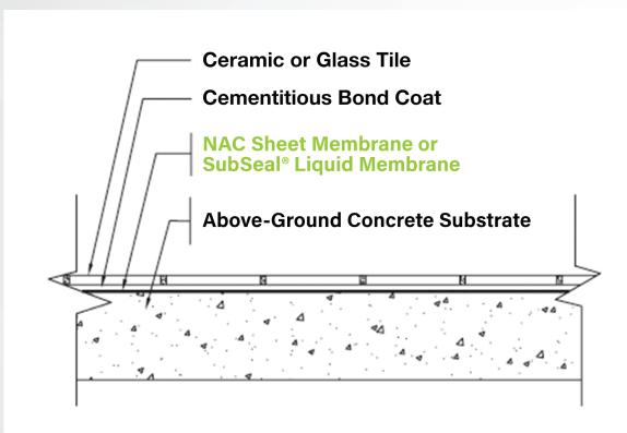
All NAC sheet membranes (ECB®, ECB® 75, Strataflex®, SAM® 3 and Super SAM® 125) and SubSeal Liquid membrane may be used for surfaces that require waterproof protection.
