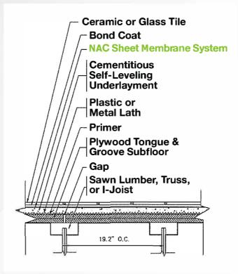
All NAC sheet membranes (ECB®, ECB® 75, Strataflex®, SAM® 3 and Super SAM® 125) may be used in this type of application for wood substrates with a cementitious self-leveling underlayment where the joist spacing is 19.2" on center.
