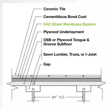
All NAC sheet membranes (ECB®, ECB® 75, Strataflex®, SAM® 3 and Super SAM® 125) may be used in this type of application for wood substrates in dry areas where the joist spacing is 24" on center or less.
