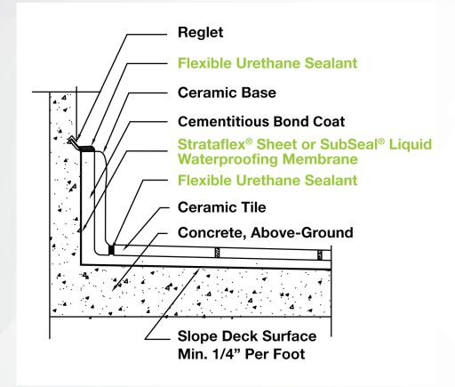
Either Strataflex sheet or SubSeal liquid membrane may be used in this application.
