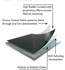
ECB Classic substantially reduces reflective cracking and delamination between the substrate and floor surface. Full floor coverage with 36" ECB Classic will provide crack isolation protection for up to 3/8" lateral substrate movement. The peel-and-stick membrane must be applied with an NAC Primer and as soon as it is positioned, flooring can be installed immediately, minimizing down time and labor cost.
