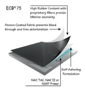
ECB 75 substantially reduces reflective cracking and delamination between the substrate and floor surface. Full floor coverage with 36" ECB 75 will protect against 1/4" lateral substrate movement. The peel-and-stick membrane is easily applied with an NAC Primer and as soon as it is positioned, flooring can be installed immediately, minimizing down time and labor cost.
