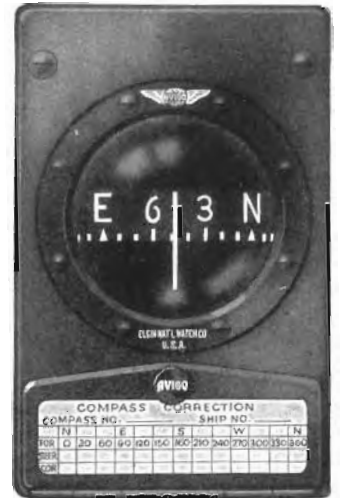
ELGIN AVIGO COMPASS. Designed to meet the demand for a compact, light-weight, reliable instrument. Many features may be attributed to the general acceptance of this compass. Bowl is spherical perfect. Design is carried to completion with a magnifying window, inside surface concave on a radius identical with the inside surface of the bowl. Card is of phenolic composition and pivoted at exact center of bowl; pivot is of highest grade steel properly hardened and polished. Cup jewel is genuine sapphire. Damping liquid is a special oil highly refined, colorless, odorless and acid free. Shock absorber high grade springs with felt cushions interposed between bowl and mount. Correction card holder attached to compass. Materials are of highest grade throughout. Phenolic composition used throughout for all major parts. Elgin Avigo Compass.....each $50.00
