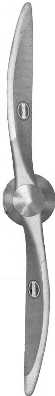
SPORT SENIORS. For engines from 90 to 115 horse power. Light alloy, adjustable blades. Range in diameters from 7' 0" to 8' 4". Weight complete with hub and puller nuts, 35 to 37 pounds.
