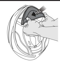
Locate the emergency labeling on the neck roll. Simply reach under the neck roll and grab the release strap, pull at a 45° degree angle towards the front of the helmet. The cheek pads will easily release from the helmet. This system should only be used by a trained medical personal.
