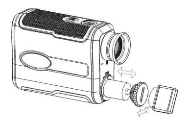
I.2 Eyepiece cover: this eyepiece is foldable, suitable for users without (graphic 1) and with (graphic 2) eyeglasses.
