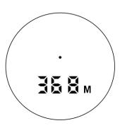
In this mode, the rangefinder will dismiss the interference of mist or rain. The shortest distance should be bigger than 25m (>25m)
