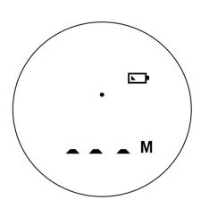
When battery power is too low, the low battery icon will appear all the time to remind user to change battery.
