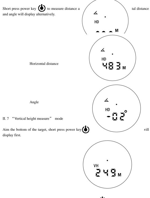
And then aim the other end of the target, short press power key to get distance and angle to the other end of target. Then vertical height will be calculated and displayed.
