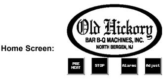
This screen is your HOME screen. This allows you to start preheating your oven, check for any alarms and adjust your cooking parameters. Pressing stop on this screen will do nothing.
