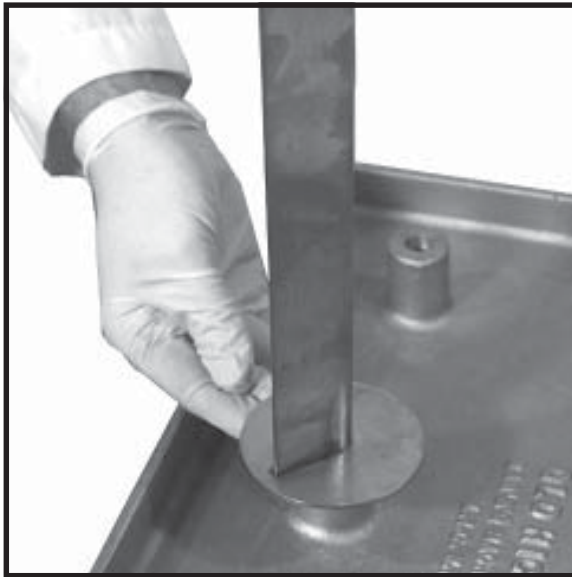
Figure 10. Using the Angle Spit
