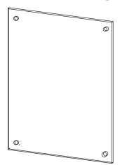
Using one the Acrylic Frame (A) panels as a template mark & drill (2) or (4) 5/16" holes in the wall.
