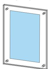
On a flat surface align and center the graphic onto one of the Acrylic Frame (A) panels and sandwich the second Acrylic Frame (A) panel over the graphic.
